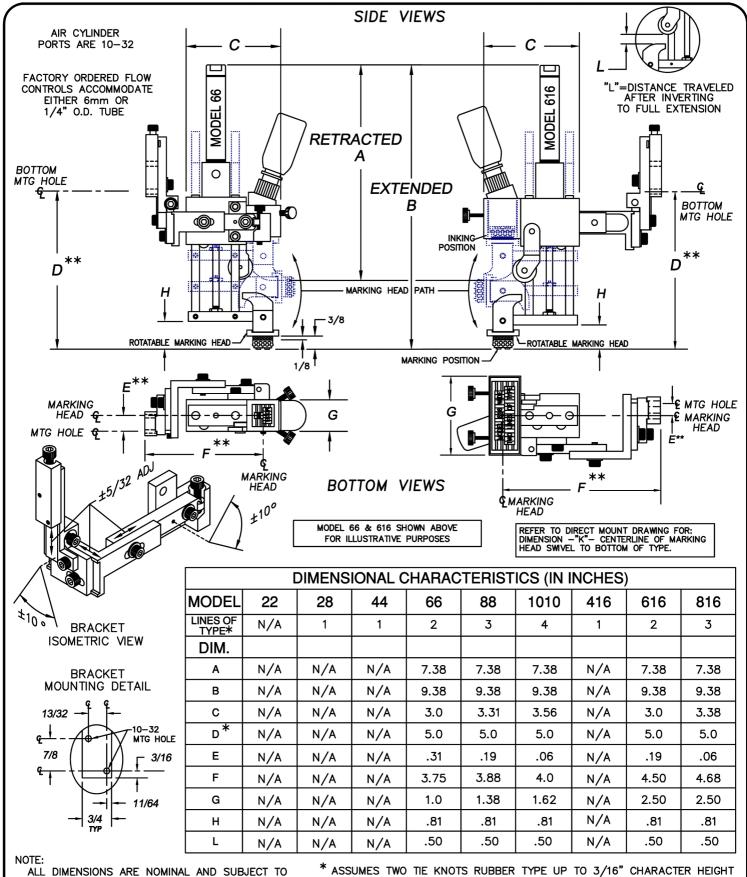
ALL DIMENSIONS ARE NOMINAL AND SUBJECT TO \* ASSUMES TWO TIE KNOTS RUBBER TYPE UP TO 3/16" CHARACTER HEIGHT STANDARD MANUFACTURING/ASSEMBLY TOLERANCES \*\* DIMENSION IS NOMINAL TO CENTER OF ADJUSTMENT RANGE FOR EACH AXIS
